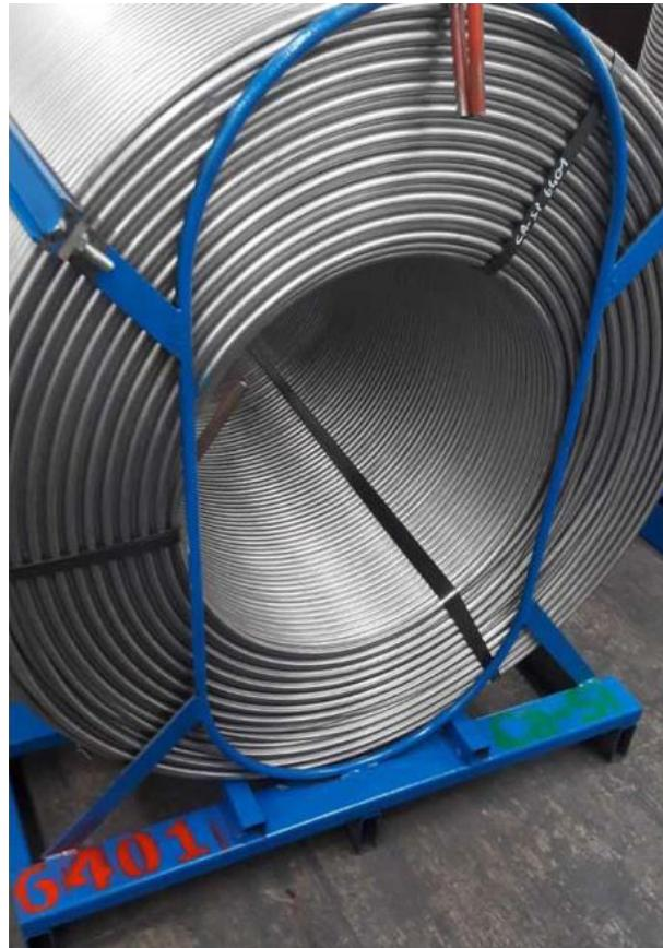
**Ca Cored Wire** The pure calcium cored wire is mainly used for Al-killed steel. Due to its low density, low boiling point and high oxidability, calcium needs to be released near the ladle bottom in order to have the best recovery. Calcium is used to transform alumina into low melting point calcium-aluminates, avoiding nozzle clogging as well as to control the shape of oxide and sulfide inclusions.
